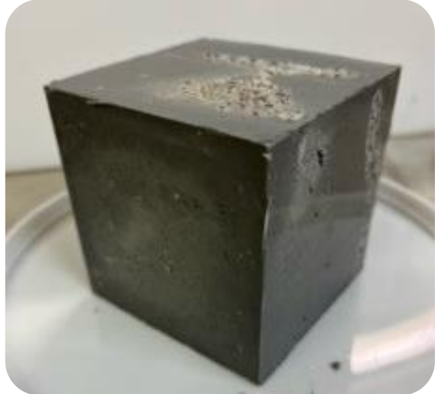
MALLETT™ encapsulated AW500 zeolite, encapsulated with pour-on technique and vibrated for 5 minutes
