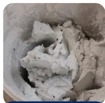
Magnesium Hydroxide sludge
