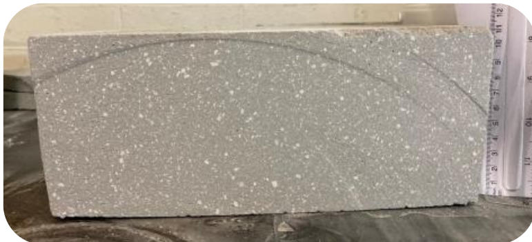
MALLETT™ encapsulated Magnesium Hydroxide sludge simulant (70:30 MgOH:MALLETT™)
