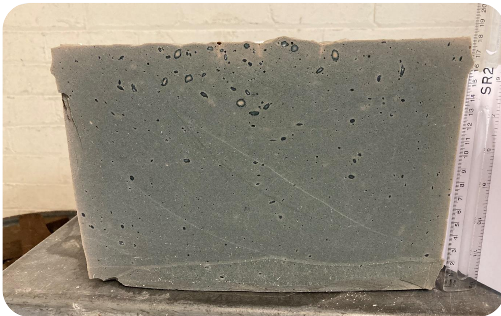
MALLETT™ encapsulated Oil simulant cross section (60:40 Oil:MALLETT™)
