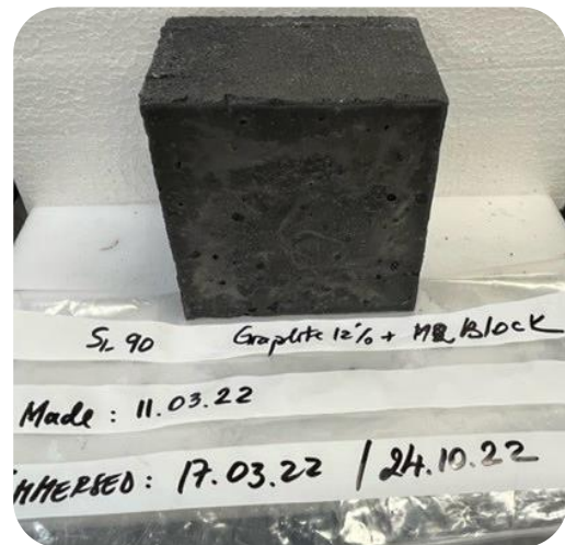
An M2 Graphite block was encapsulated with 12% w/w graphite powder, and immersed in deionised water for 7 months, with no cracking or deterioration visible
