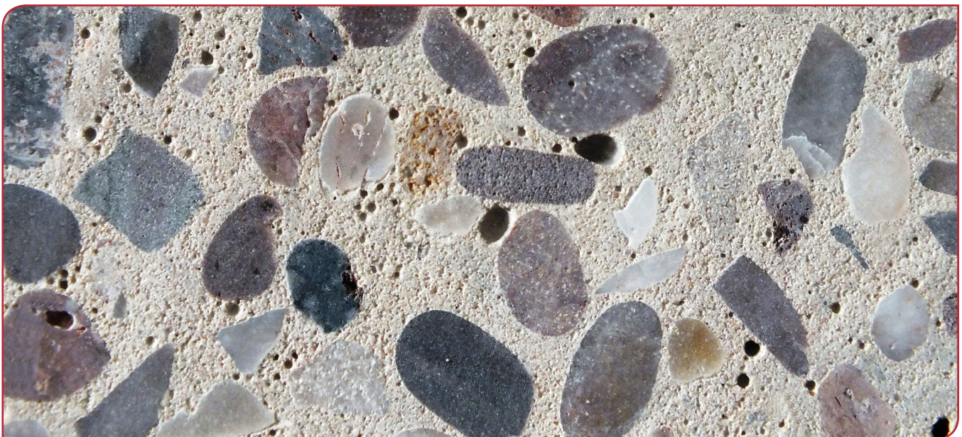
Below: MIDAR terrazzo is GGBS concrete with decorative aggregate. Ground surface gives a terrazzo effect.
